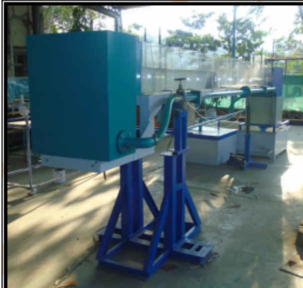
Tilting Flume (5m Long)
