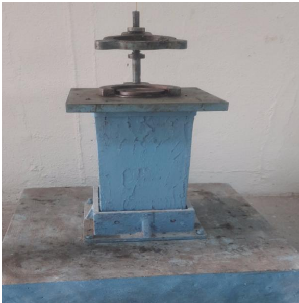
Marshall Stability Test Apparatus Application: Sample Compactor
