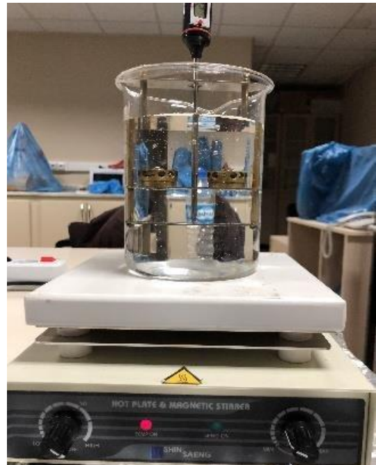
Softening Point Test Application: Softening Temp.
