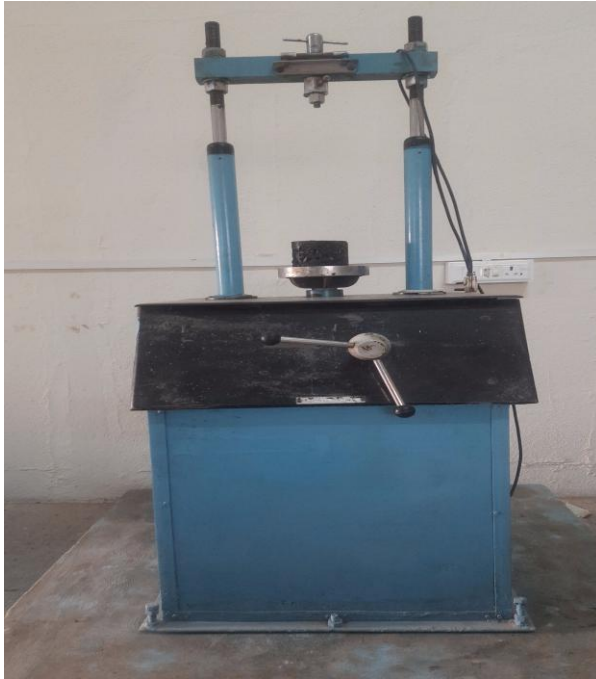
Marshall Stability Test Apparatus Application: Bitumen Mix Samples
