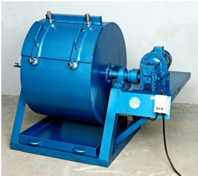
Los Angeles Testing Machine Application: Abrasion Test
