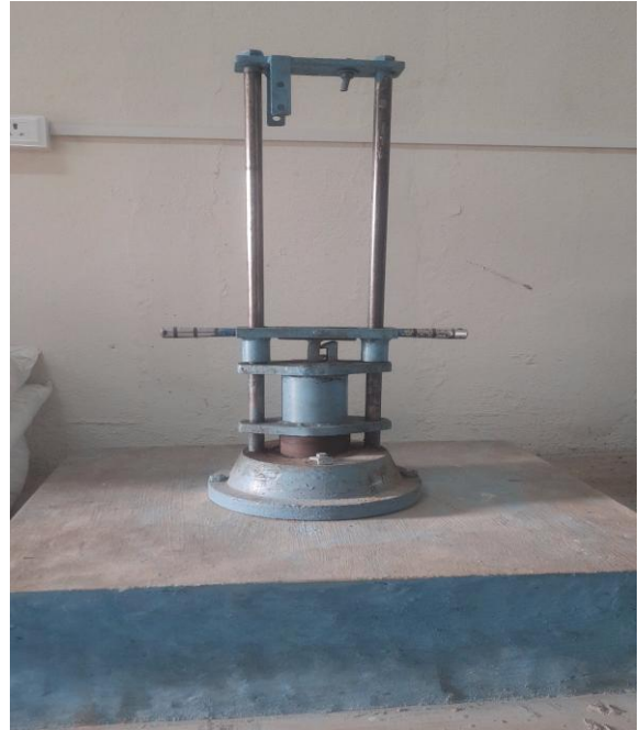
Impact Test Apparatus Application: Test toughness of Aggregate
