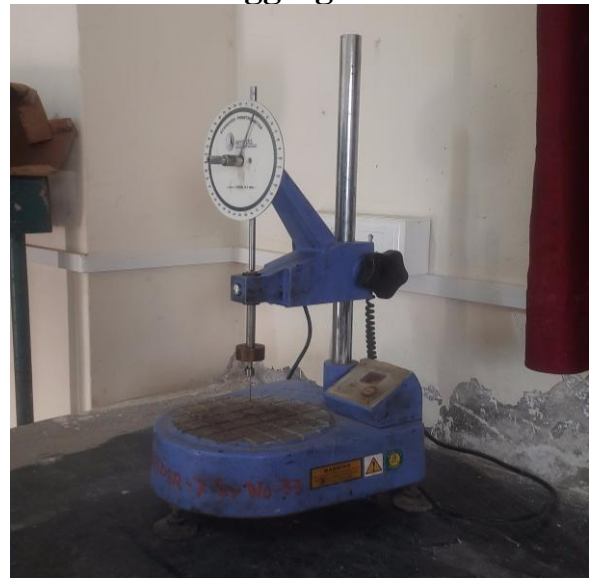
Penetrometer Application: Test Bitumen Grade
